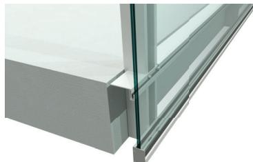
Fill the gap by using the L profile, which is done at the same time as other profile mounting.
